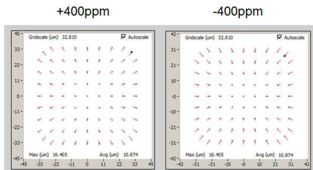
**Fig. 4.** Vector map showing available magnification and scale adjustment over an 84mm diameter lens field
