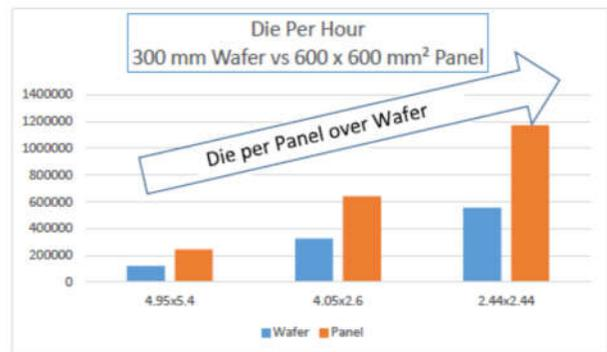
**Fig. 8.** Productivity increase that can be expected when processing on 600 x 600mm<sup>2</sup> panel over 300mm diameter wafer
