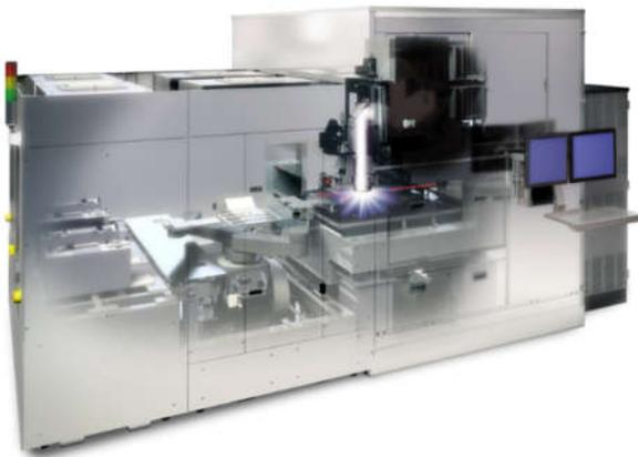
Fig. 2. JetStep® S3500 Panel Lithography System
