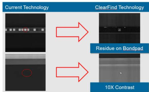
**Fig. 9.** Fluorescence solution: highlights organic residues on metal and array
