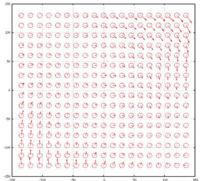
Fig. 3. Vector map of die placement offset on a reconstituted panel (Note: Circle radius =  $4\mu\text{m}$ )
