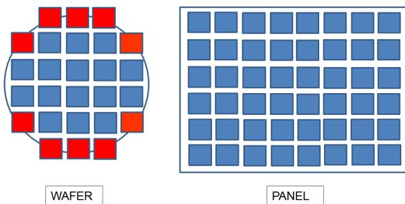
**Fig. 7.** Illustration of partial die exposure on a wafer compared to die exposure on a panel, non-productive areas of die on wafer shown in red
