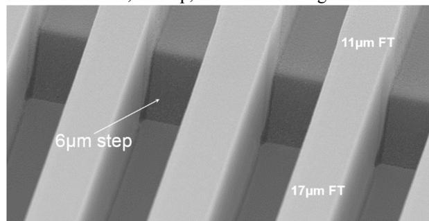
**Fig. 6.** Photoresist image of RDL over topography
