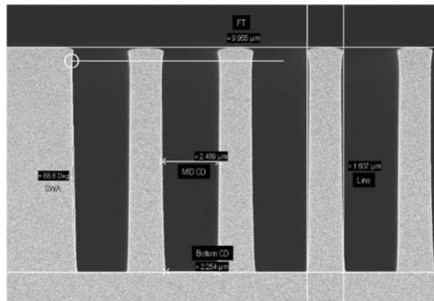
**Fig. 5.** 5:1 Aspect Ratio,  $2\mu\text{m}$  RDL
